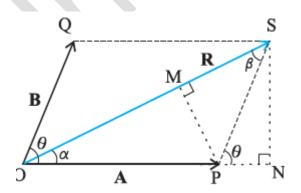
**Solution**: Let OP and OQ stand for the two vectors A and B that form a q-angle .Then, using the vector parallelogram approach, OS also stands for the resultant vector R.
