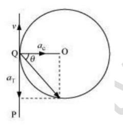
Assume the cyclist starts from point P and rides toward point Q. At point Q, he uses the brakes and reduces the bicycle's speed by  $0.5m/s^2$ . This acceleration is parallel to the tangent at Q and in the opposite direction of the object's motion.
