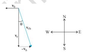
her is the velocity of rain relative to the velocity of the bicycle she is riding. That is  $v_{rb} = v_r - v_b$ . It is given by:
