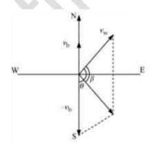
The angle between  $v_w$  and  $(-v_b) = 90^\circ + 45^\circ$
