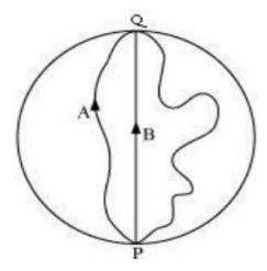
**Solution**: The smallest distance between a particle's initial and final coordinates determines displacement. In the example, all of the girls begin at point P and work their way to point Q. Their displacements will have the same magnitude as the diameter of the ground.
