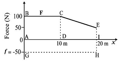
Figure shows a plot of the applied force. At x = 20 m,  $F = 50 \text{ N} (\neq 0)$ .
