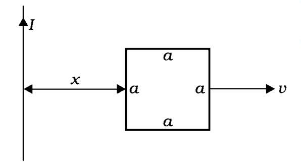
Ans: (a) Insert a small element dy in the loop, y distance from the long straight wire. magnetic flux=dy,  $d\phi$  =BdA B is the magnetic field at y.
