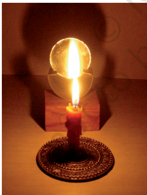
Fig. 11.16 Virtual image formed by a concave mirror
