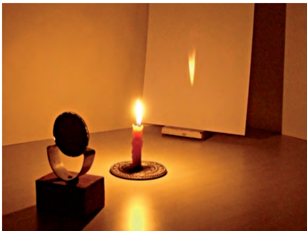
Fig. 11.15 Real images formed by a concave mirror
