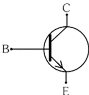
The above figure shows the circuit symbol of a transistor. Select the correct statements given below:
