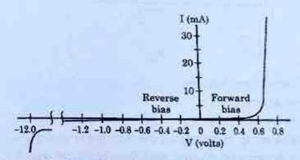
Estimate the dynamic resistance of diode at V = -0.6 volt.
