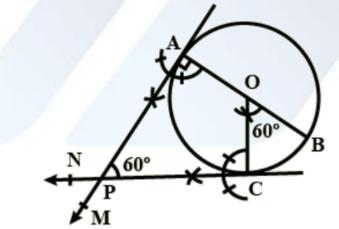
Draw a Circle: Use a compass to draw a circle with radius 3 cm and center 0. Draw Two Radii: Mark a point A on the circle and draw OA. Using a protractor, mark a 60° angle at 0 and draw OB.
