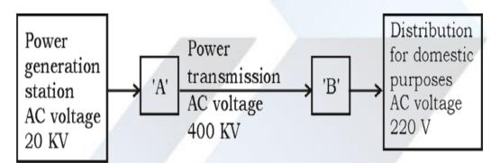
Name the devices to be used in the places indicated as ' *A* ' and ' *B* '.
