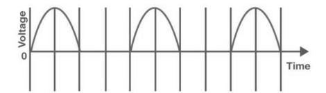
b. The diode functions as a rectifier in the circuit and allows only the positive voltage cycle to flow through the circuit, thus blocking the negative cycle. This results in a pulsating DC output, where only the positive half of the AC cycle is allowed through, and the negative half is blocked.
